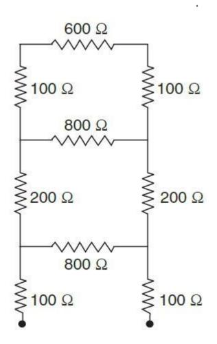
4-b. In the circuit of Fig. , find the current through each resistor using nodal 4 analysis.(CO1)
