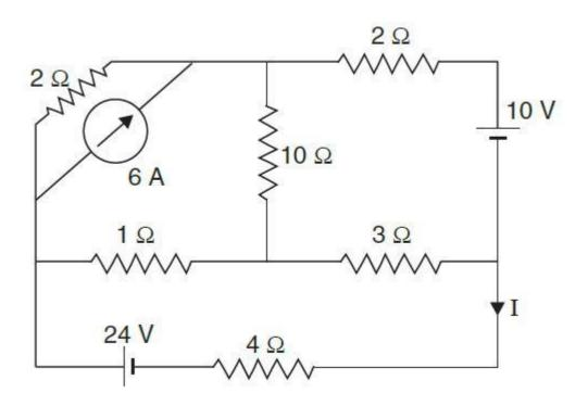
3-b. Find thevenin voltage, thevenin resistance and the load current flowing 5 through load resistor in the circuit below using Thevenin's Theorem.(CO2)
