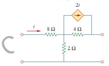
7-b. Write the Reciprocity condition in Y and H Parameters. For the ladder network in 10 Fig, determine the Y parameters in the s domain. (CO4)
