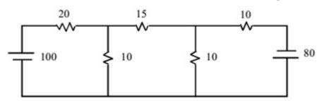
4-b. Find the current through various resisters using nodal analysis. (CO1)
