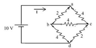
4-b. Find the current  $I_x$  and  $V_x$  in the circuit using Norton' Theorem. (CO1)
