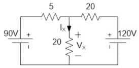
3-b. In the network shown in Figure , determine the value of load resistance load resistance to give maximum power transfer and the power delivered to the load. (CO1)
