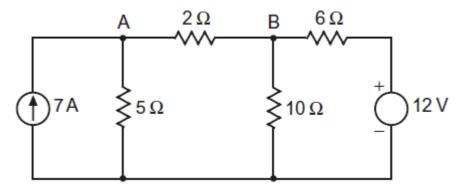
4-b. Using mesh equation method, find current in the resistance  $R_1$  of the network 10 shown in Figure (CO1)
